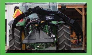
Butt Plate The butt plate enables the grapple to bunch logs and piles, and prevents logs from damaging the tractor when being picked up.
