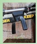
Heel Bar The heel bar enables light logs to be lifted and stacked, prevents logs from getting hung up on the frame, and keeps logs in line while skidding.
