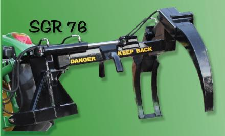
VALBY SGR 76 Tractor Grapples are built using a bypass design whereby the single tine on one side of the grapple passes through the gap between the double tines on the opposite side of the grapple. The tines tighten up completely on the load, keeping it balanced and in control. The result is that logs are easily picked up and rolled in. The SGR 48 is designed for lighter duty work, and accomplishes the same task using one tine on each side.
